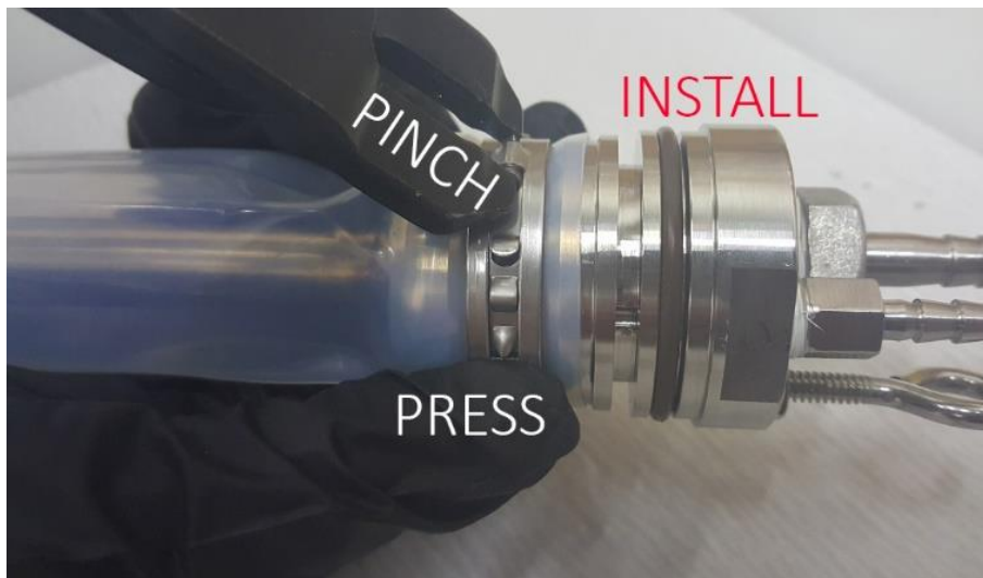
Figure 4-4: Installing the Bladder Clamp
