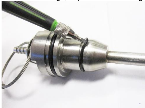
Figure 4-5: Removal of O-rings
