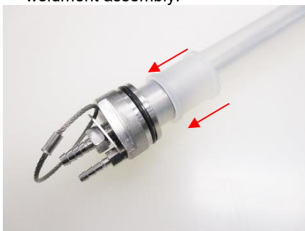
Figure 4-14a: Compression Ring on Bladder
