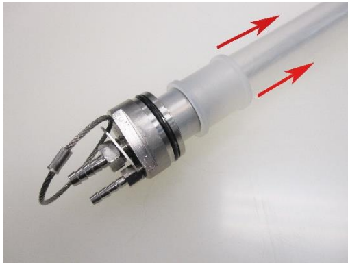
Figure 4-3: Removal of upper Compression Ring
