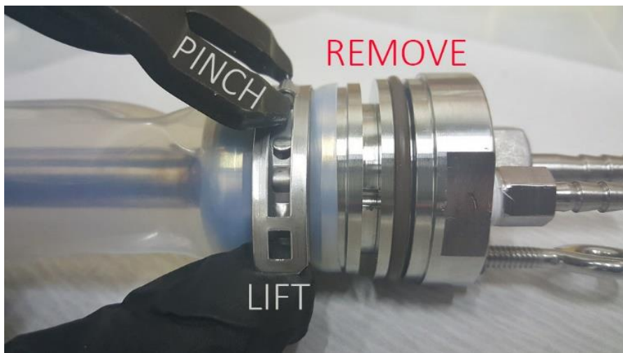
Figure 4-2: Removing the Bladder Clamp
