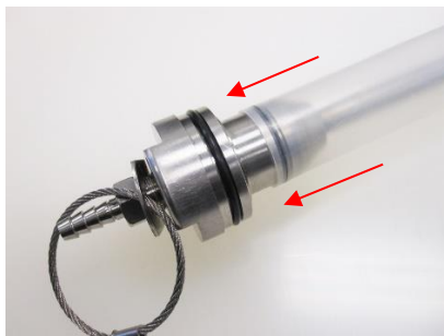
Figure 4-13a: Sliding bladder on
