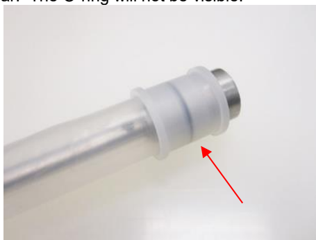
Figure 4-15: Bottom Compression ring with visible O-ring
